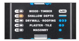
By selection of an appropriate scale, the instrument can also be used for the detection and location of elevated moisture in or behind a range of covering materials such as wall, floor and ceiling tiles, siding, carpet and laminated floor coverings.
