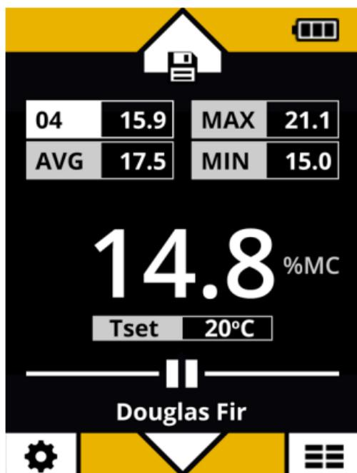
The Professional PTM 2.0 can save up to 100 readings in its memory from any of the 3 Modes – Wood, WME (Ref) or Drywall.
