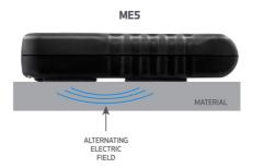
As there is a wide variation in the nominal electrical impedance of different material types, the instrument is provided with five selectable scales which are optimized for testing
