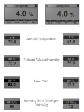
To change temperature between °C and °F and the Humidity Ratio between g/kg and grains/lb, press the Double button to go the Main Menu; scroll down and select 'TEMPERATURE SCALE' with the Double button, scroll and select with the Double button; and press the Double button to return to the main screen.
