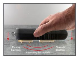
This field penetrates the material under test. The very small alternating current flowing through the field is inversely proportional to the impedance of the material. The instrument detects this current, determines its amplitude and thus derives the moisture value.
