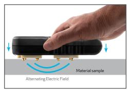
Instrument pressed on to material surface to measure/detect moisture
