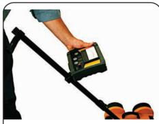
6. Clip the Control Panel Meter onto the meter bracket.
