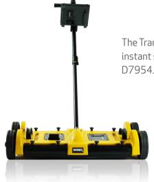
The Tramex Dec Scanner is a mobile non-destructive impedance scanner designed for the instant surveying of moisture conditions in roofing and waterproofing systems per ASTM D7954.
