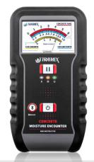
The Tramex Concrete Moisture Encounter 5 (CME5) is a non-destructive analog moisture meter for concrete floors and slabs providing instant and precise quantitative measurement of moisture content using Gravimetric testing as a baseline. The CME5 also provides Carbide Method equivalent readings for concrete and other cementitious substrates as well as comparative readings as per ASTM F2659.
