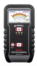
The Tramex Concrete Moisture Encounter 5 (CME5) is a non-destructive analog moisture meter for concrete floors and slabs providing instant and precise quantitative measurement of moisture content using Gravimetric testing as a baseline. The CME5 also provides comparative readings of gypsum floor screeds as well as comparative readings of concrete as per ASTM F2659.
